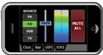
Custom control panel served on an iPhone.
